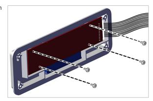
6. Separate the bezel from the touchscreen display assembly.
