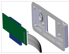
8. Carefully connect the display cable to the touchscreen display assembly.
