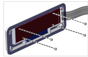
11. Secure the display bezel to the front trim using the original four (4) T10 torx screws and washers.
