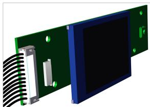
9. Place the touchscreen display assembly into the display bezel.
