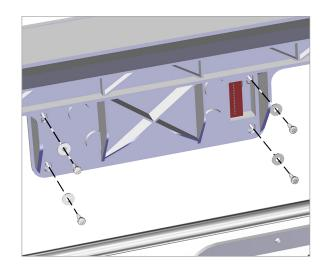
5. Loosen and remove the four T10 torx screws securing the touchscreen display assembly to the display bezel.
