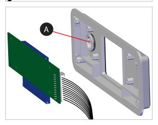
10. Secure the touchscreen display assembly to the bezel with the original four (4) T10 torx screws.
