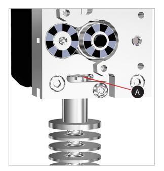
34. If the affected extruder is extruder 2, vertically center print jet 2 in the pinch clamp of the extruder housing and tighten the T10 torx screw (A) enough that the print jet is securely held. If the printer has only one print jet, vertically center print jet 1 in the extruder housing and tighten the T10 torx screw using the T10 x 60 torx driver.
