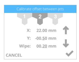
11. Referring to the illustration at the beginning of this procedure, print jet 2 needs to be increased by .3 mm. Select the value until the first digit (A) to the right of the decimal point is highlighted.
