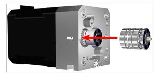
32. Align the print jet tab with the channel in the extruder. Insert the print jet into the extruder.
